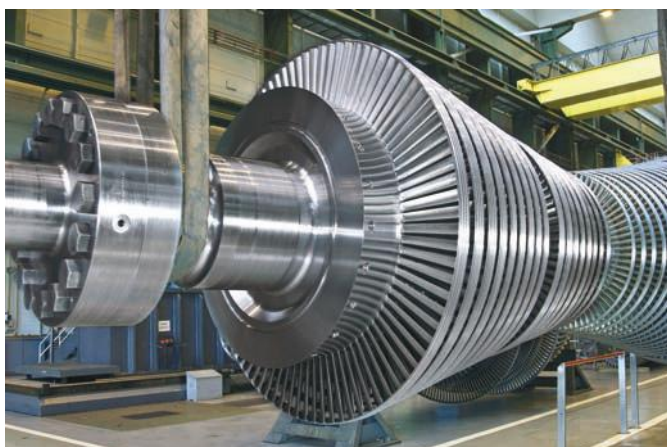
Figure 15.6 The rotor of a steam turbine
