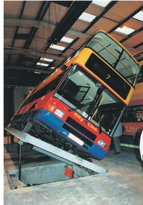
Figure 11.6b A double-decker bus being tilted to test its stability
