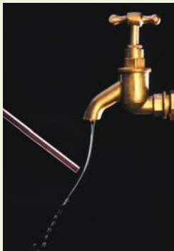
Figure 35.6b A slow stream of water is bent by electrostatic attraction.
