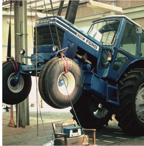
Figure 11.6a A tractor under test to find its centre of mass
