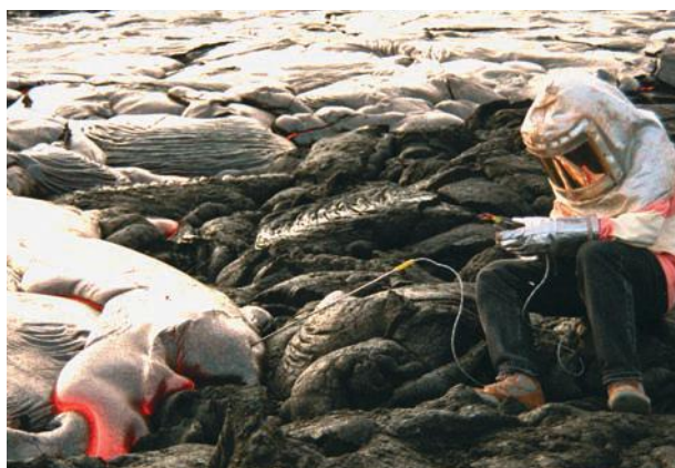
Figure 20.1 Use of a thermocouple probe thermometer to measure a temperature of about 1160^{\circ}\text{C} in lava
