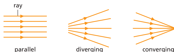
Figure 26.4 Beams of light
