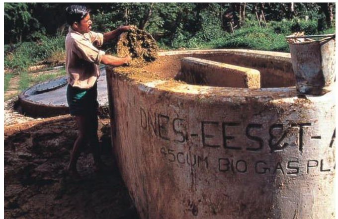
Figure 15.5 Feeding a biogas digester in rural India
