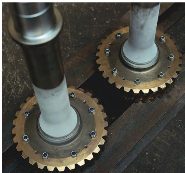
Figure 19.1 'Shrink-fitting' of axles into gear wheels
