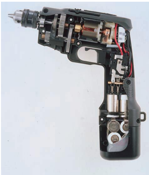
Figure 46.5 Motor inside an electric drill
