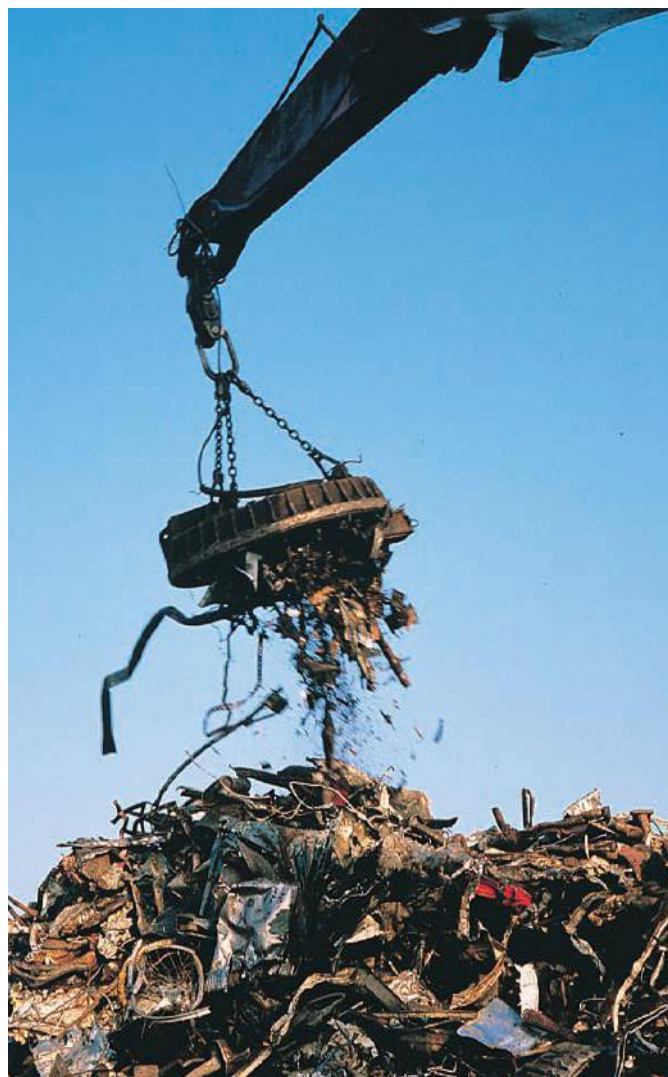
Figure 45.7 Electromagnet being used to lift scrap metal
