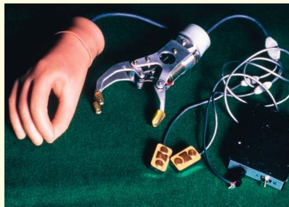
Figure 42.9 Electronically controlled artificial hands
